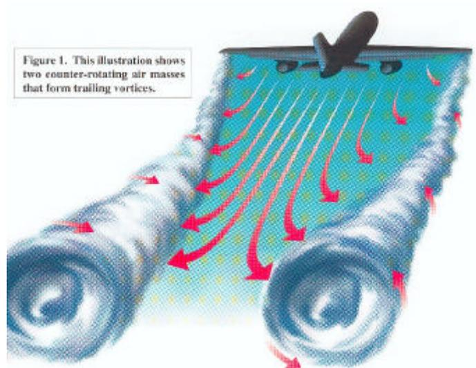
Research has shown that for a typical jet transport airplane, the wake descends behind the generating airplane at approximately 300 to 500 feet per minute for about 30 seconds. As seen in Figure 2, the descent rate decreases and eventually approaches zero at between 500 and 900 feet below the flight path.
