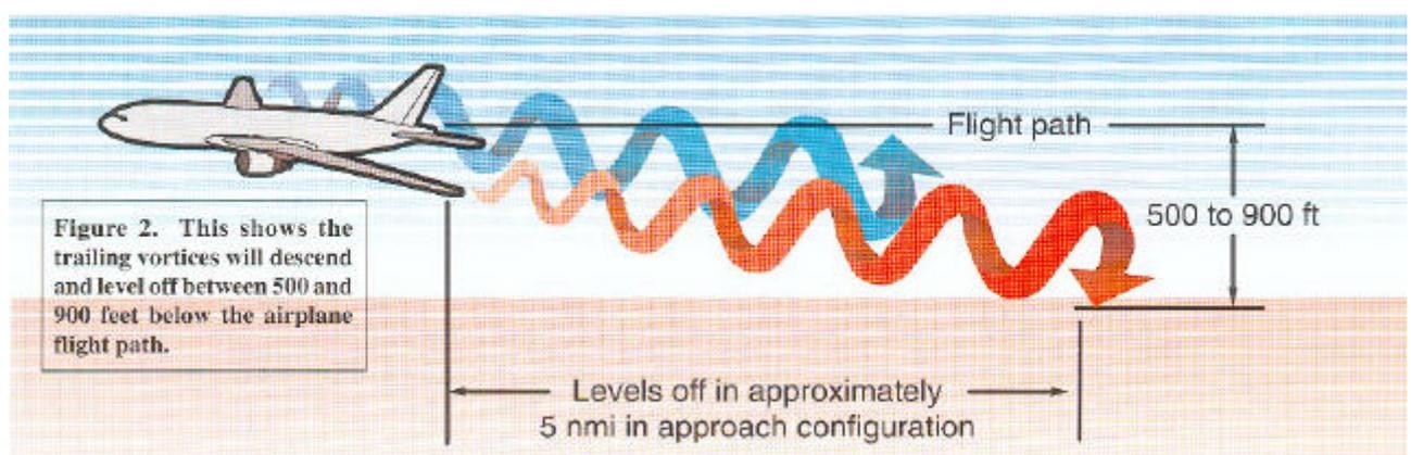
Prevailing surface winds will also influence the direction the vortices will move; thus, during parallel runway operations, the wake turbulence hazard must be a consideration on both runways. Additionally, under some crosswind conditions, vortices have been observed to "bounce" - that is, descend toward the ground and then later begin to rise up. For the conditions where bounce has been observed, the crosswinds are strong enough to clear the vortices from the approach corridor.
